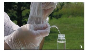
First, squeeze the full sampler just below the top to expel water resting above the flexible check valve. (Photo 1, top left)
