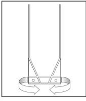
Fold the two holes at bottom of HydraSleeve together and attach weight
